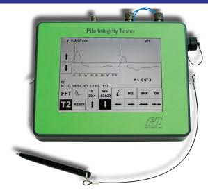
pile length. If a defect is present along the shaft, its size and location affect the propagation and reflection time of the wave.
