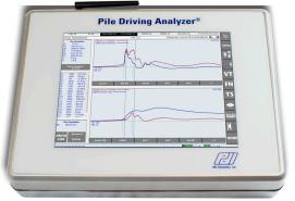
Criterion and contributes to safe and economical production pile installation. The PDA-8G calculates for every hammer blow the static soil resistance at the time of testing (by Case Method and/or iCAP®, a real-time signal matching analysis), driving hammer performance, maximum driving stresses, and evaluates pile integrity. The high-speed PDA-8G data transmission allows testing at hammer operating blow-rates as high as 120 bpm, without loss of data.
